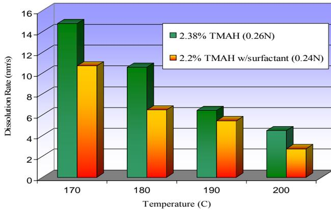
Figure 3 – Dissolution Rate at various LOR soft bake temperatures with different developer concentration (normality)
