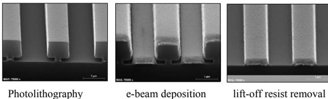
**Figure 7** – Bi-layer lift-off metallization sequence
