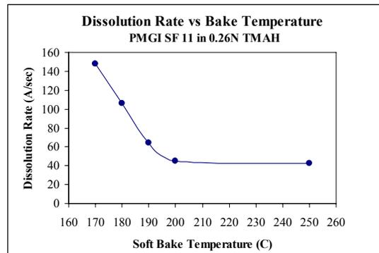
Figure 6 – Dissolution rate vs. bake temperature through the glass transition temperature
