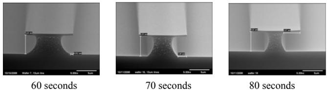
Table 2 – Spray Develop Profiles for thick LOR - increasing develop time with constant wafer spin-speed
