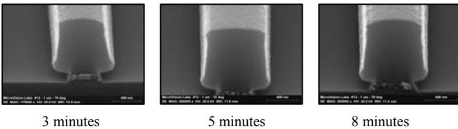
Table 4 – Develop profiles for thin LOR - increasing soft-bake time at constant soft-bake temperature
