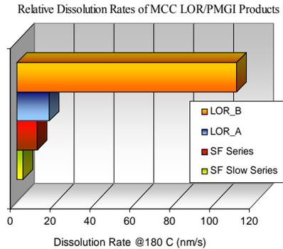
**Table 5** – Dissolution Rate for a 1 μm film soft baked at 180°C for 5 minutes
