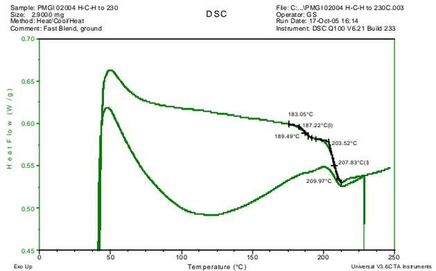
Figure 5 – Glass Transition Temperature (Tg) of PMGI
