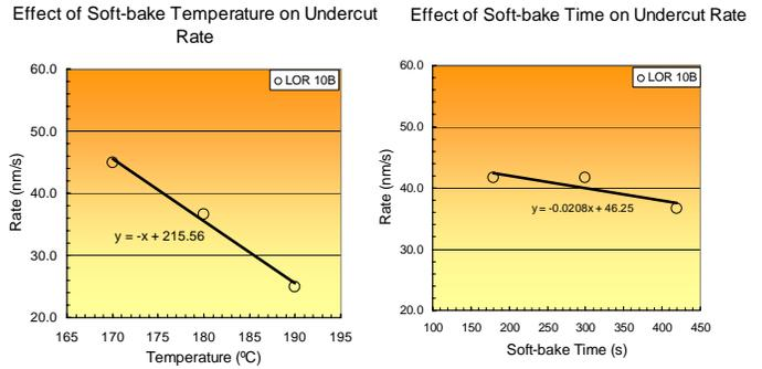
Figure 4 – Comparison of soft-bake temperature versus soft-bake time for a 1 μm LOR film
