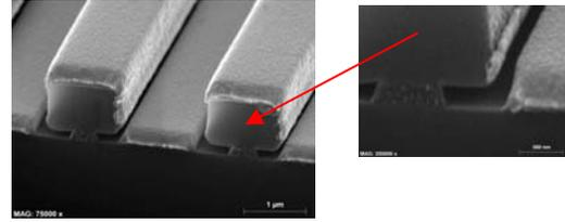
**Figure 8** – Bi-layer lift-off in e-beam metallization of gold – discontinuity in the deposited metal allows for complete lift-off removal of resist
