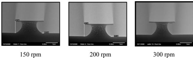
Table 1 – Spray Develop Profiles for thick LOR - increasing wafer spin-speed with constant spray time
