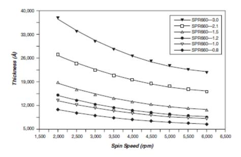
Figure 3. Spin Speed Curves—Dyed SPR660 Photoresist
