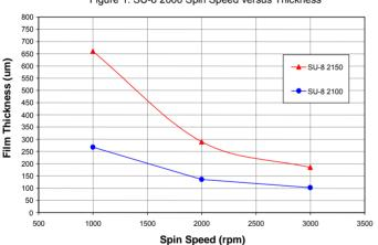
Figure 1. SU-8 2000 Spin Speed versus Thickness
