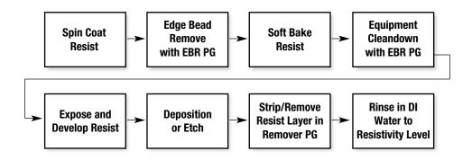
The edge bead removal process is equipment and substrate specific. Therefore, the following baseline process suggestions may be modified and optimized after considering the following:
