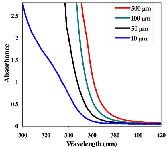
Figure 2. SU-8 Absorbance vs. Wavelength for Various Film Thicknesses
