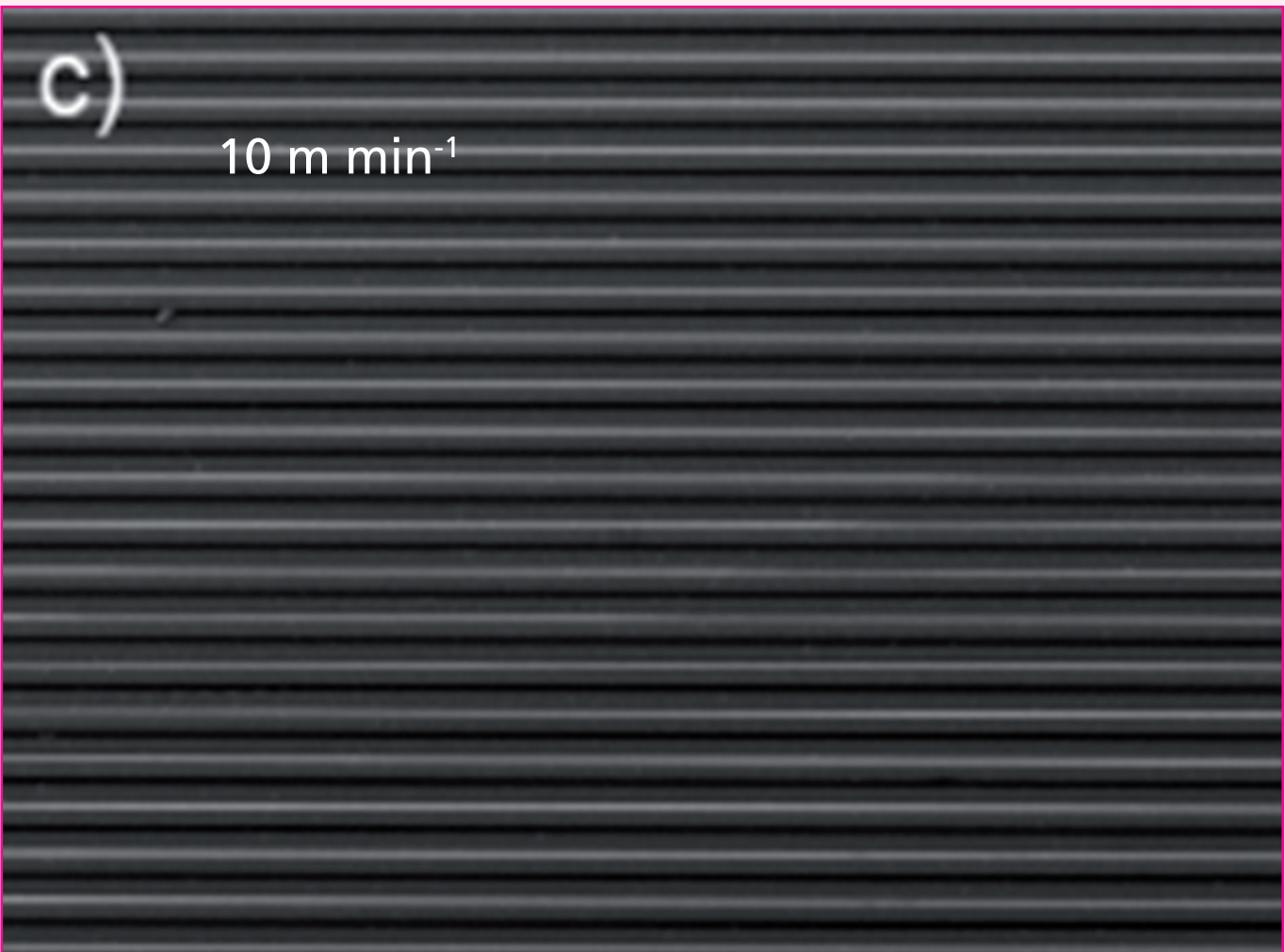
R2R-NIL with mr-UVCur26SF: SEM images after variation of the web speed, substrate PET foils, room temperature gravure coating, SAM fluorinated Ni roller molds, Hg bulb radiation for curing (Courtesy of Joanneum Research Materials, Austria).
