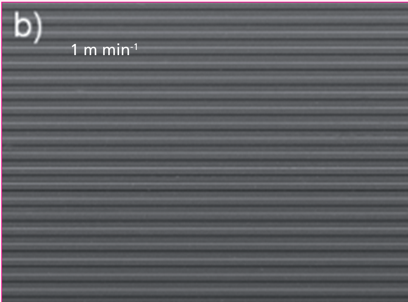
R2R-NIL with mr-UVCur26SF: SEM images after variation of the web speed, substrate PET foils, room temperature gravure coating, SAM fluorinated Ni roller molds, Hg bulb radiation for curing (Courtesy of Joanneum Research Materials, Austria).
