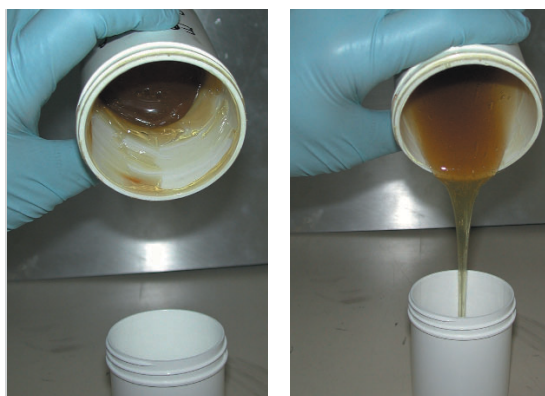
Figure 11: Highly thixotropic epoxy hardener. Material does not flow (left) until it is stirred for a few seconds (right).
