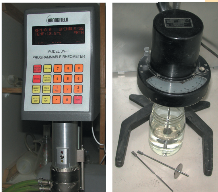
Figure 12: Two types of viscometers (left) cone and plate viscometer and (right) spindle viscometer.
