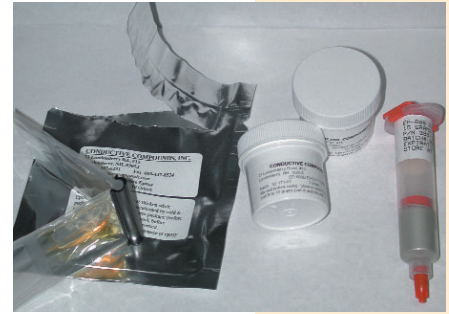
Figure 3: Packaging options for two part epoxy adhesives. From left, (a) plastic pouch with resin and hardener weighed out and separated by a removable plastic clip. (b) Plastic open top containers with the exact amounts of resin and hardener. The end user adds the hardener to the resin container and mixes them. (c) Pre-mixed/frozen syringes that must be stored at -40 degrees C.
