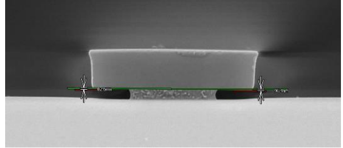
Figure 2 - Post SiO 2 stably constructed bi-layer 9 \mu\text{m} L/S
