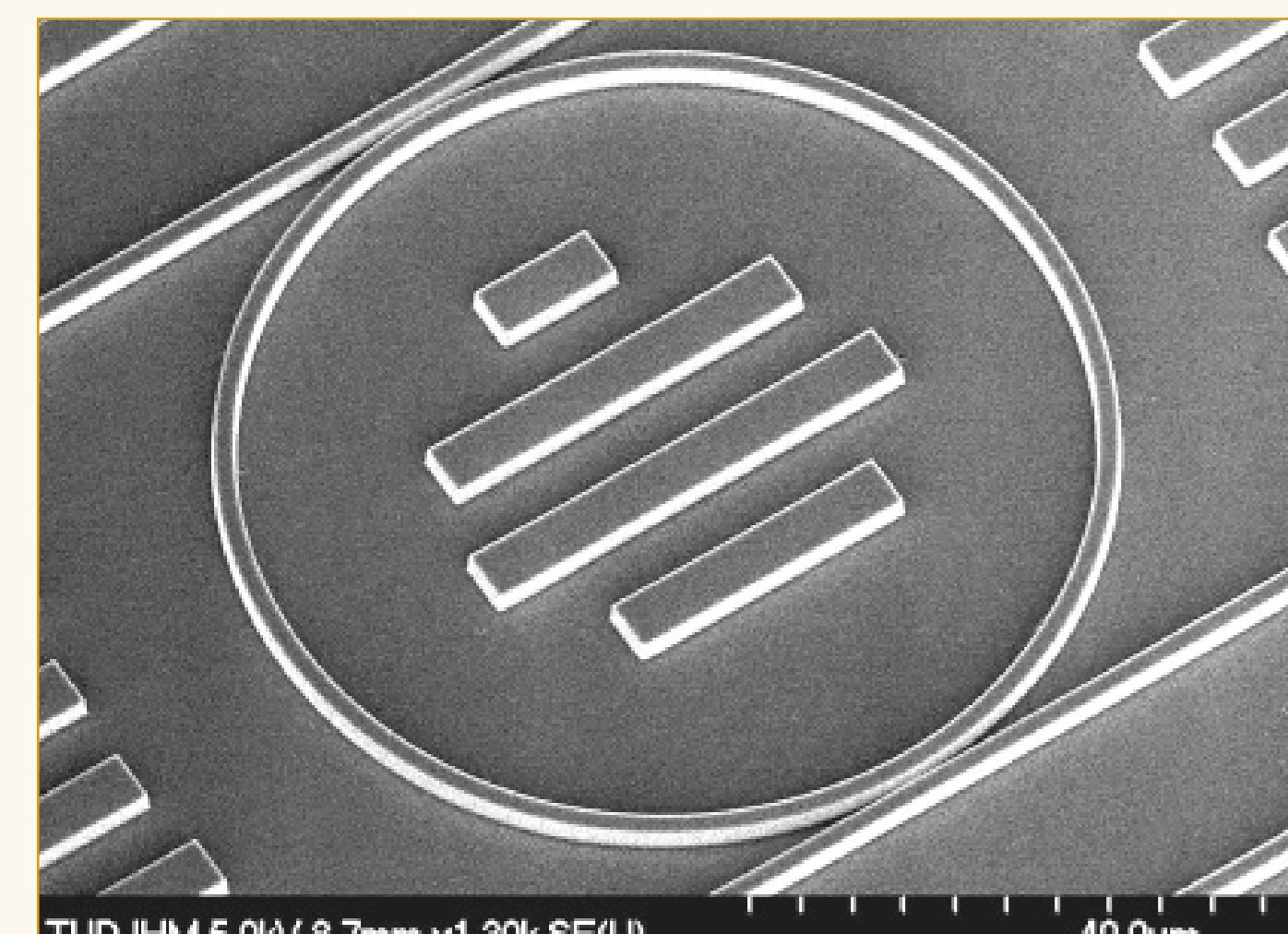
Replicated OrmoCore microring resonator
