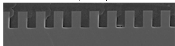
Figure 7 LOR C - 10 \mu\text{m} Deep Trench Filling with 5 \mu\text{m} Line/Space
