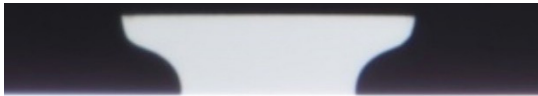
Figure 2. 30 \mu\text{m} line with shallow undercut, using sample processing conditions (see Table 2) with 1 minute of development .
